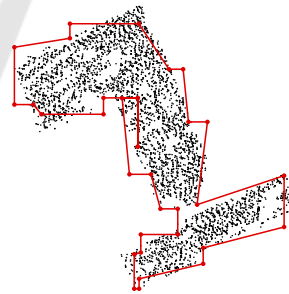
Figure 5: The shape represented by the point is actually tilted by \approx 25^\circ against the x -axis. Not accounting for this initial orientation yields unpleasant results.
