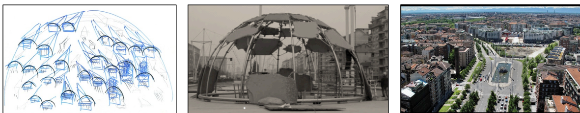
Figure 2: Merz's igloo fountain in Turin: design, construction, final.
