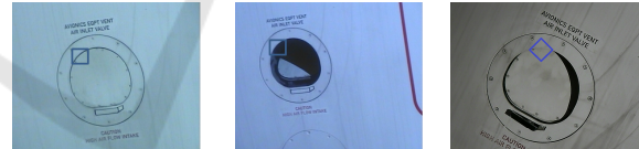
(a) Closed vent (negative). (b) Open vent (positive). (c) Partially open vent (positive).
