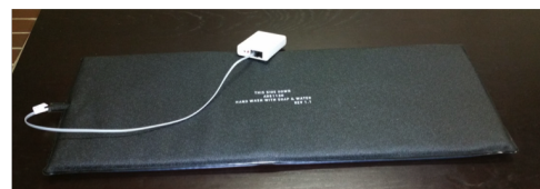
Figure 2: Self-calibrating mat sensor, for under-the-mattress positioning.
