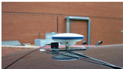
Figure 4: GPS + IMU module set up on IVVI 2.0 roof.
