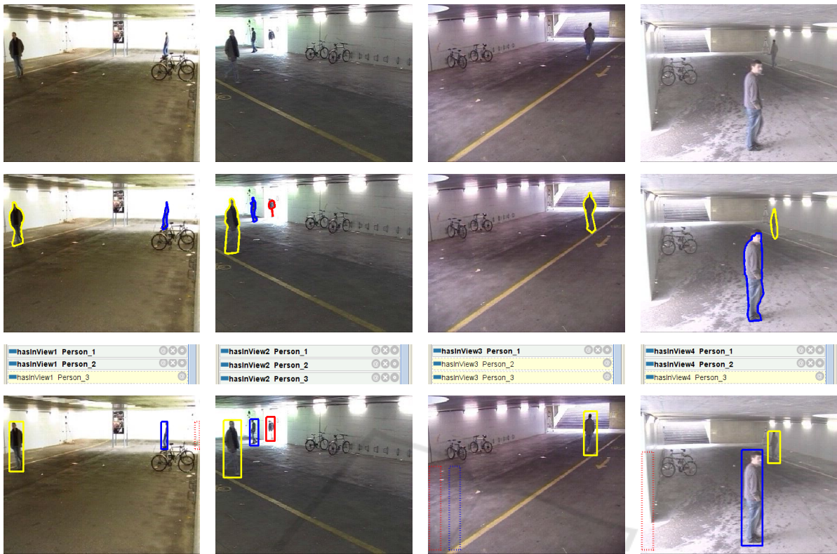
Figure 4: Examples of results obtained with our approach for a scene captured by four synchronized cameras with overlapping field of views. First column: view 1; Second column: view 2; Third column: view 3; Fourth column: view 4. First row: step 1 - raw data images. Second row: step 3 - visible persons detected in each of the camera views (e.g. Person 1 by yellow active contour; Person 2 by blue active contour; Person 3 by red active contour). Third row: step 6 - snippet of the automatically generated description for each view (extracted knowledge in blue, inducted knowledge in yellow). Fourth row: step 7 - detected persons in all views (bounding boxes), including the hidden persons (dotted bounding boxes). Best viewed in color.
