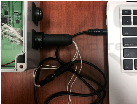
Figure 15: Audio to sensor channel adapter.
