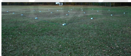
Figure 17: Hammer shock test deployment.
