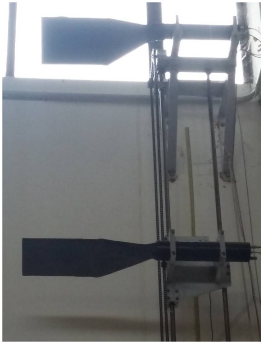
Figure 3: Experimental setup: adjustable distance scintillation counters, lightguides, photomultiplier, high-voltage supply and signal cables.
