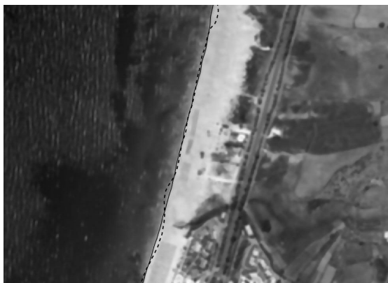
Figure 8: The waterline differences between 2003 and 2010. The dashed line refers to 2003 image, while the solid line refers to 2010 image from Google Earth.
