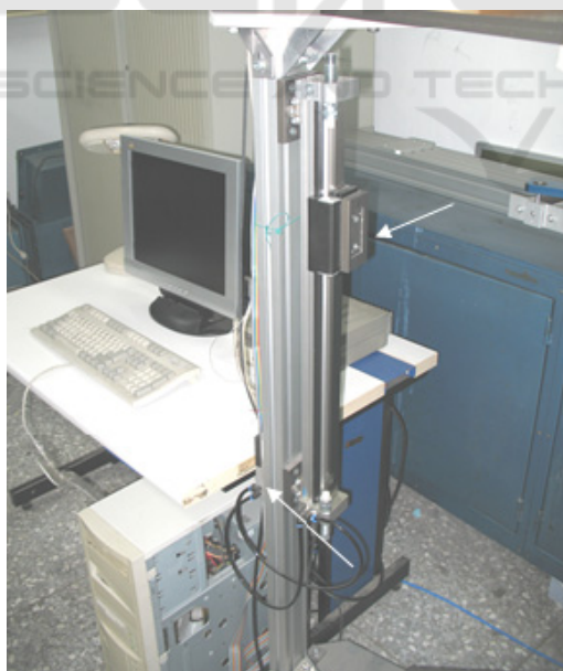
Figure 1: Rodless pneumatic actuator system.
