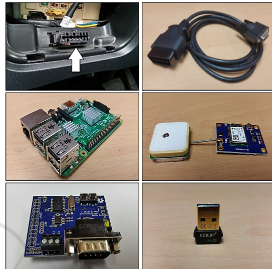
Figure 4: OBD (II) Interface (Top Left), OBD Cable (Top Right), Raspberypi2 (Middle Left), NEO-6M GPS Module (Middle Right), SKPANGS PICAN board (Down Left), WIFI Module (Down Right).
