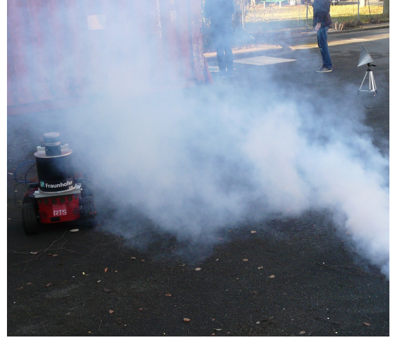
Figure 5: This figure shows the setup of the experiment. It has been performed in a yard with a robotic platform, which is equipped with the 2D MPR and a 3D Velodyne VLP-16 LiDAR.
