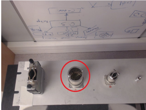
Figure 4: View from the gripper camera during the first attempt of the first test. The operator had to unplug the circled connector.
