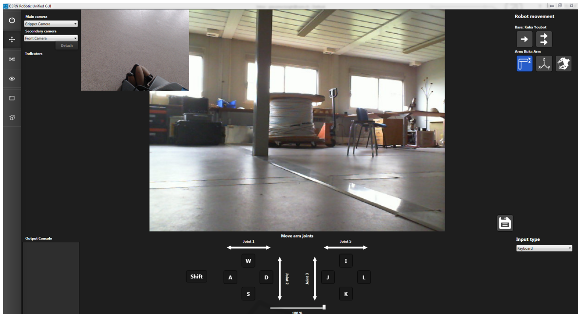
Figure 2: Control window of the Graphical User Interface connected to a robotic platform equipped with a robotic arm and two cameras, with the keyboard as a selected input device.
