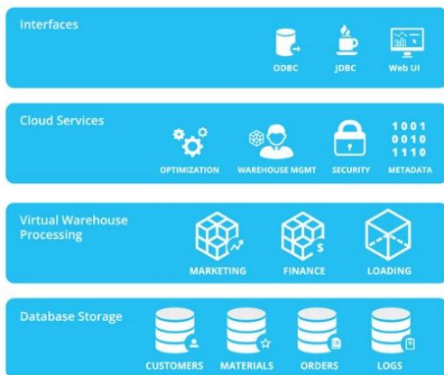
Figure 5: Snowflake logically integrates the storage and computing but there is physical separation (Snowflake).
