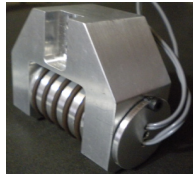
Figure 5: Friction-based tangential force sensing device fitted with torque sensor.
