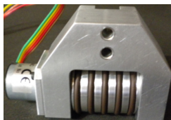
Figure 7: Encoder fitted to the roller assembly.
