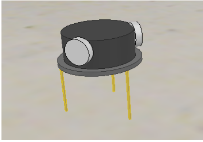
Figure 1: Graphical visualisation of the Kilobot robot in V-Rep simulation software.
