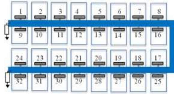
Figure 3: Placement of tilesets with their ID number on the U-shaped transmission line.
