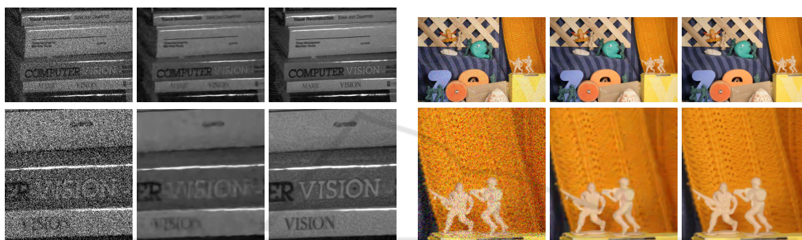
Figure 2: For each of the examples, first row, from left to right: noisy frame, VBM4D, SPTWO. Second row: details of the previous images. We display the noisy and denoised central frames of the sequence. The standard deviation for the gray book sequence is 50, and for the color army sequence is 30. The errors for the results on the gray sequence are: VBM4D (RMSE=6.34), SPTWO (RMSE=4.77); and for the color sequence: VBM4D (RMSE=7.35), SPTWO (RMSE=7.01). This figure illustrates the ability of the white noise removal algorithm in (Buades et al., 2016) compared to the state of the art VBM4D (Maggioni et al., 2011).
