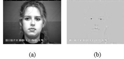
Figure 3: Symmetry transform image. (a) Grayscale image; (b) Corresponding symmetry transformation. Darker regions correspond to areas that have a high circular symmetry.
