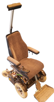
Figure 3: The experimental setup consists of a Kinect time-of-flight camera mounted on an electric wheelchair.
