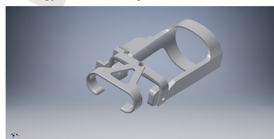
Figure 6: Mechanical prototype for wrist flexor/extensor tremor suppression.
