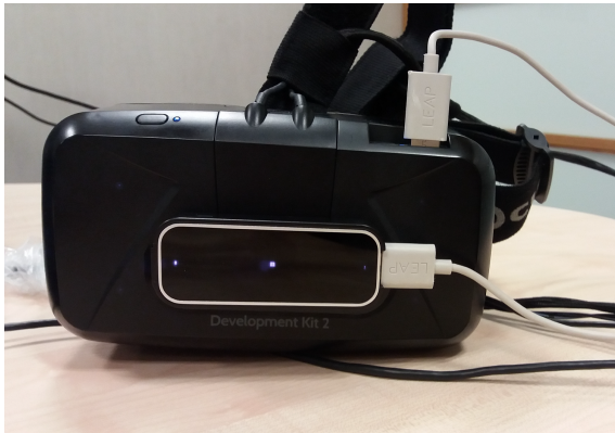
Figure 9: Leap Motion can be attached to the Oculus Rift in order to provide gesture recognition of the user's hands.
