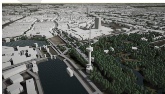
Figure 6: Euromast tower in Rotterdam, the Netherlands. It consists of multiple geometry elements using the “building:part=yes” tag.
