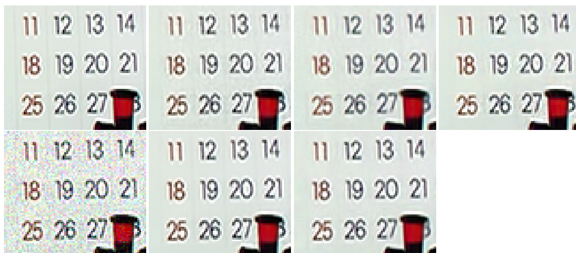
Figure 5: Results of denoising for mobile (zoom on frame 37, noise 20). Top: ground truth, NL-Bayes local, BM3D local, VBM4D; bottom: Noisy, NL-Bayes global and BM3D mix.
