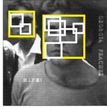
Figure 7: The yellow englobing rectangles of detected faces include one or several facial LBP-appearance regions represented by white rectangles.
