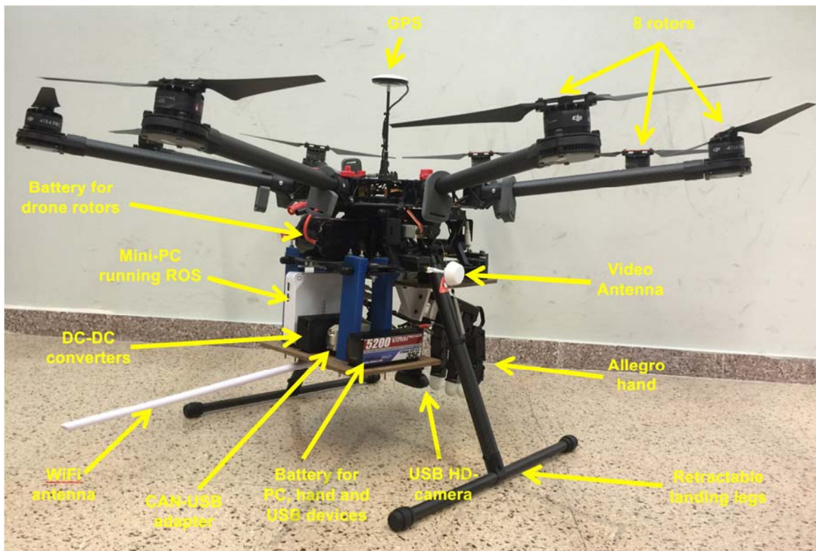
Figure 2: Main additional equipment added to the drone.
