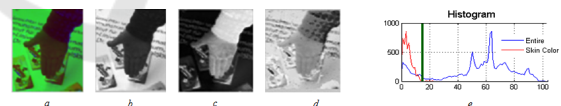
Figure 3: Skin Color Segmentation in Complex Background of Image from Treisch’s Data-set a. Input Image b. ‘L’ color component c. Color component ‘a’ d. Color component ‘b’ e. Histogram of Skin and Entire Image.
