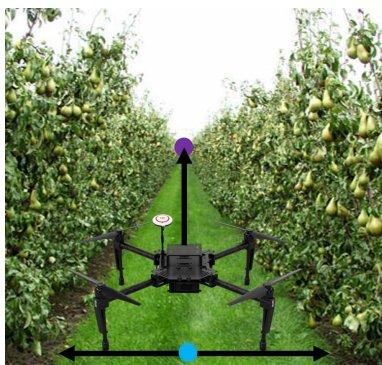
Figure 2: An example of an orchard. Blue point is the CP of corridor and purple point is the VP of the corridor.
