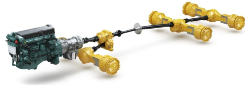
Figure 2: Drivetrain in a Volvo A40G Articulated hauler.
