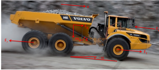
Figure 1: Longitudinal forces acting on an articulated hauler.
