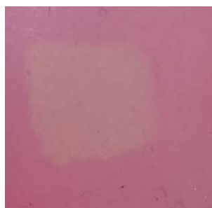
Figure 2: PMMA/MEH-PPV blend image after 45.50 hours of irradiation exposure.
