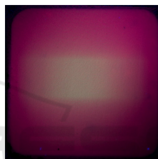
Figure 5: Luminescence of (\text{Ba}_{0.5}\text{Sr}_{0.5})_2\text{SiO}_4:\text{Eu}^{3+} (red emission) and (\text{Ba}_{0.5}\text{Sr}_{0.5})_2\text{SiO}_4:\text{Eu}^{2+} (green emission) after x-ray exposure.
