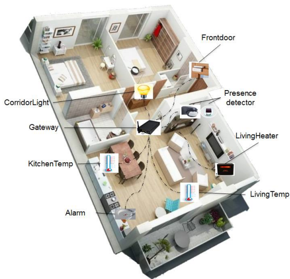
Figure 1: Alice’s smart home equipped with various devices, interacting through a centralised gateway.
