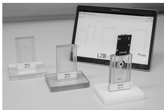
Figure 2: Sensor system with circuit board and data acquisition/transfer via Bluetooth 4.0 for the concentration of pC 3, pC 2 and pC 1.
