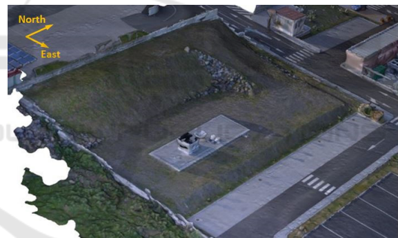
Figure 2: The 3D textured mesh of the landslide-like area recreated by the mapping software.
