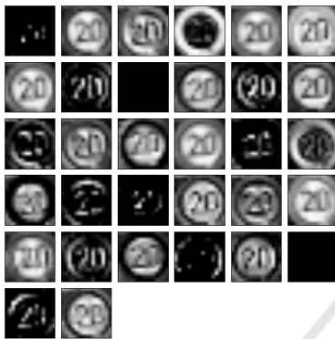
Figure 5: Second Layer: Max Pooling.
