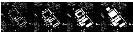
Figure 6: Evolution of the geodesic reconstruction (iteration from 1 to 185).
