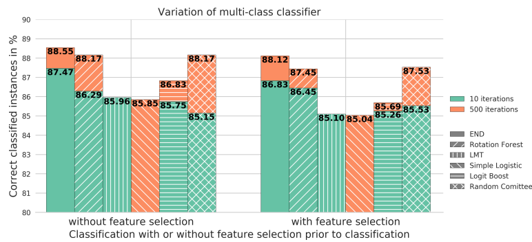
Figure 4: Benchmarks of best performing classifiers in a multi-class setup using implementations of Weka with default parameter settings and 10-fold cross-validation, but adjusted iterations to 10 and 500 iterations. The LMT algorithm has a self-optimized number of iterations, the exact number is unspecified. Simple Logistic is by default well-tuned and uses 500 iterations. Feature selection prior to classification shows no significant impact.
