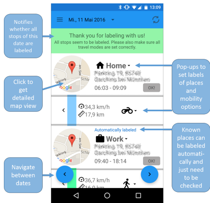
Figure 1: Our self developed Mobility Companion App for Android based smartphones used for ground truth data collection. The timeline view shown of identified stops for selected date extended with labeling possibilities for places and transportation modes.
