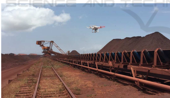
Figure 7: Simulated inspection with an UAV over a real production environment.
