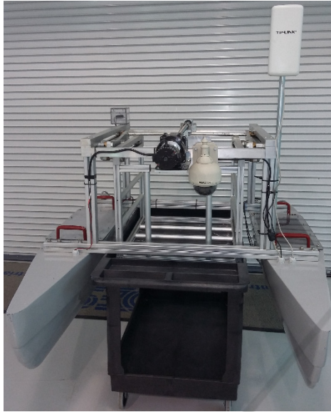
Figure 6: USV developed at CIDESI, mounted in a carriage for ground transportation.
