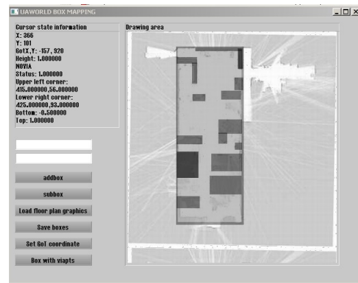
(a) 2D top view of interior obstacles included as Axes Parallel Boxes in map design area of prototype design application.
