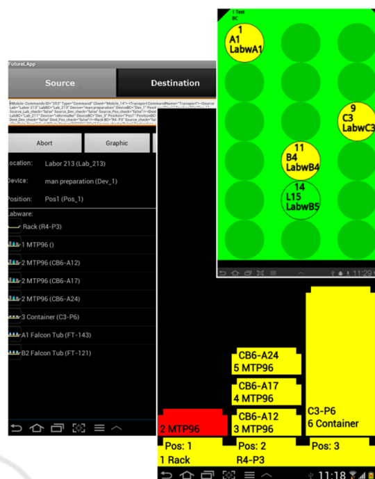
Figure 5: Screenshot of the mobile device list and graphical user interface with the required transport arrangement of the labware.
