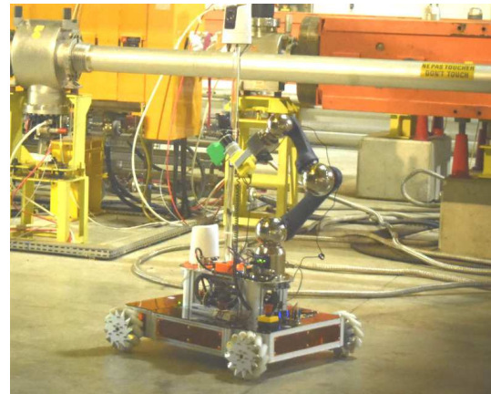
Figure 1: Robot developed at CERN for surveying tasks.
