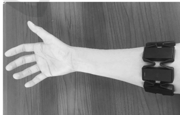
Figure 3: Positioning the sensor for signals acquisition.
