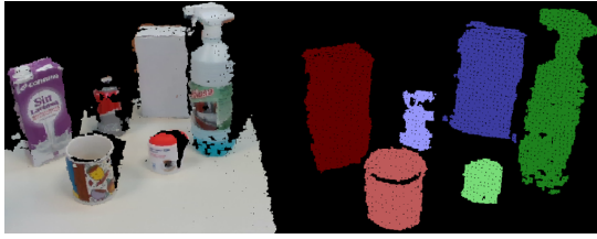
Figure 2: Scene segmentation. (left) original registered point cloud, (right) detected objects after plane segmentation and clusters detection.
