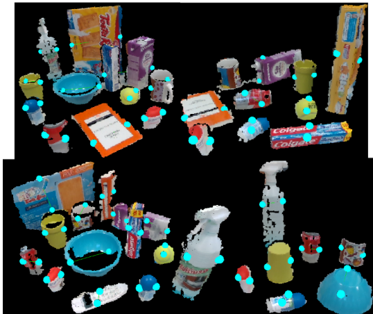
Figure 6: Samples of grasps proposed over clutter scenes. Top: (left) Mix12-a, (right) Mix10-a. Bottom: (left) Dataset-b, (right) Cyl-sphere.
