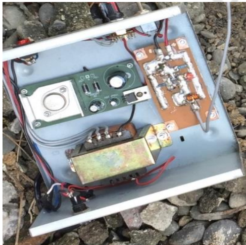
Figure 2. Transmitter and power supply modules
