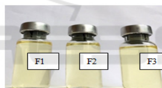
Figure 2: Appearance of the prepared sunscreen nanoemulsion (F1, F2, F3) containing avobenzone and octyl methoxycinnamate after storage for 12 weeks at room temperature
