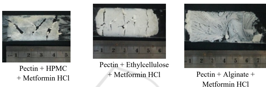
Figure 3: Polymers of pectin, alginate, HPMC and ethyl cellulose (two polymers combination) can not form film membranes with Metformin HCl
