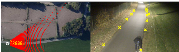
Figure 1: World position of camera (white), field of view (red) and calibration points (yellow) sprayed on the ground and measured with high precision GPS.
