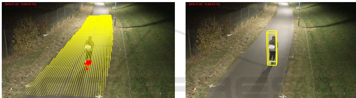
(a) Sampling grid and classifier scores. Yellow indicates low scores and red high scores.
