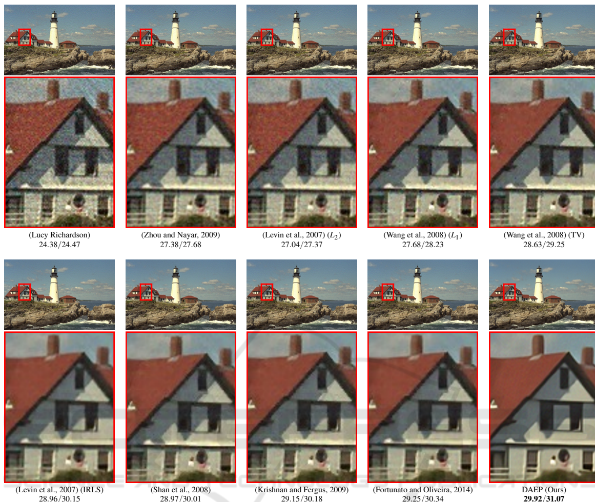
Figure 6: Comparison of non-blind deconvolution methods on the 21st image from the Kodak image set (Kodak, 2013). For each method, we report the PSNR ( dB ) of the visualized image (left) and the average PSNR on the whole set (right). The results of other methods were reproduced from Fortunato and Oliveira (Fortunato and Oliveira, 2014) for ease of comparison.
