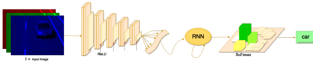
Figure 1: Proposed CRN model. First, the three channels input image is processed through a series of convolutions and pooling. Then, after reaching the fifth stage, we flatten the resulting set of features into a single high-dimensional representation \phi(I) \in \mathbb{R}^f . Finally, we feed the feature vector to the LSTM that learns the corresponding class label.
